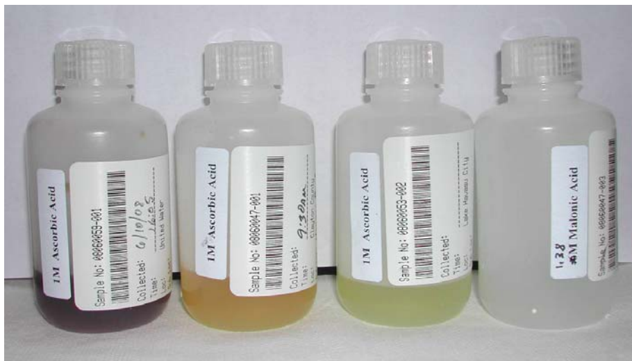
Figure 2.3 Quenched hypochlorite samples from utilities using ascorbic acid (left 3 bottles) and malonic acid (right bottle)
